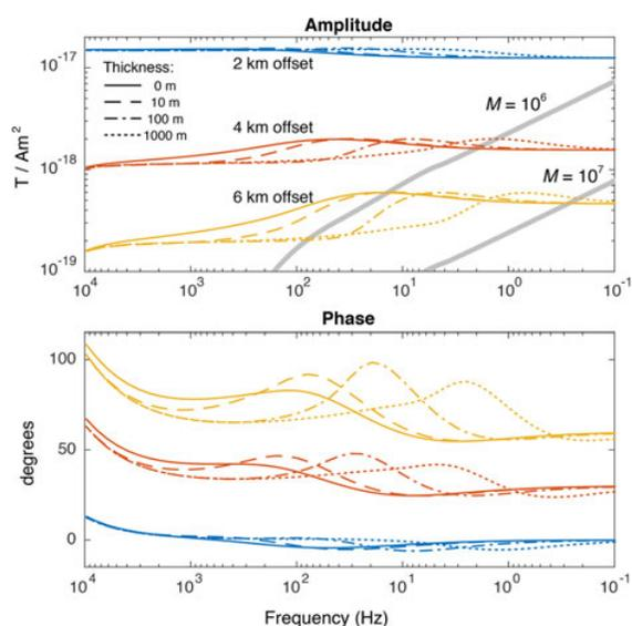
**Fig. 6.** FDEM responses for the test model shown as a function of frequency at various offsets from the transmitter loop. The various thin colored lines show the responses as a function of conductive layer thickness. Phase values for 4 and 6 km offsets have been shifted by 30 and 60° for visual clarity. Thick gray lines show approximate vertical magnetic-field noise levels  $B_{noise}$  for two stacking moments. See text for further discussion of the noise levels.
