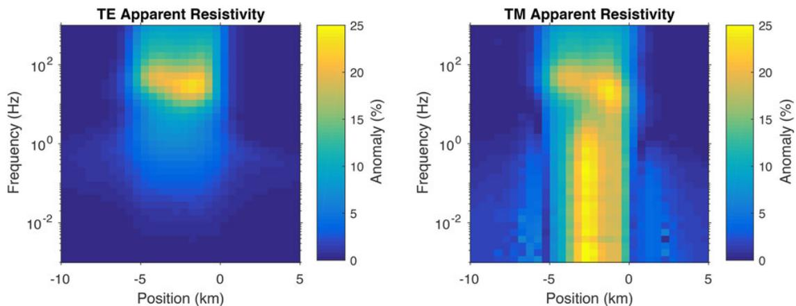
**Fig. 14.** Relative anomaly in the MT responses due to the 1 m thick seawater intrusion at –5 to 0 km lateral position. The anomaly is calculated by taking the relative difference in the response from models with and without the seawater intrusion and is shown as a function of frequency and receiver position.
