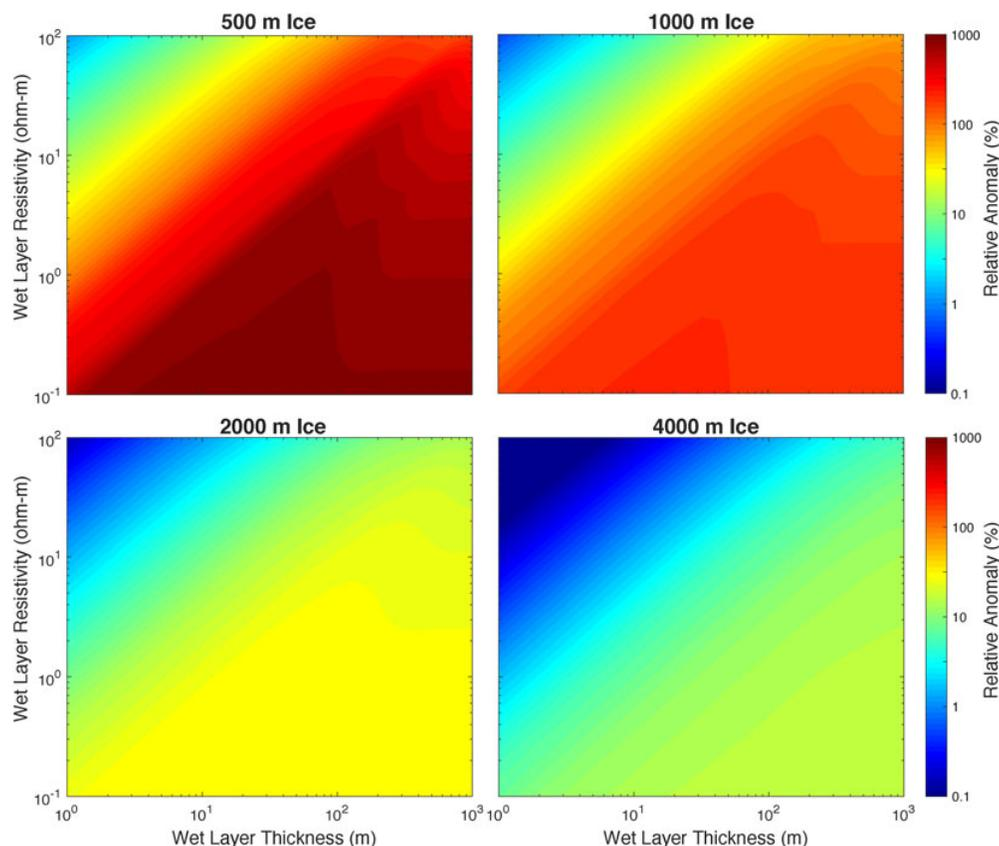
**Fig. 7.** Relative anomaly in the FDEM response for a model with a conductive wet layer shown as a function of variable layer resistivity and thickness. The anomaly is computed as the maximum relative difference between the response of the wet layer model and the response from a model without the wet layer. The maximum relative difference was computed in the frequency band 0.1–10 000 Hz at offsets from 2 to 6 km and is shown for four different ice thicknesses (500, 1000, 2000 and 4000 m).
