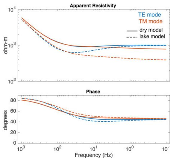
**Fig. 11.** Transverse electric (TE) and magnetic (TM) apparent resistivity and phase MT responses for a receiver located at the center of the lake in our SLW-like domain (lake model) and in a similar model with the lake removed (dry model).
