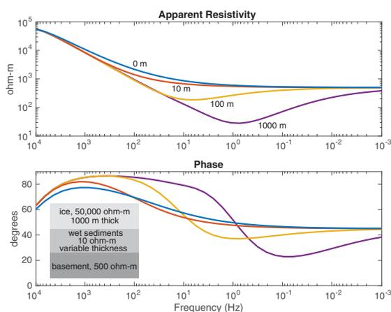
**Fig. 3.** Effect of a subglacial conductive layer on the MT response for a 1D model with 1000 m thick resistive ice overlying 10  $\Omega$ -m wet sediments of variable thickness, as indicated by the labeled curves.
