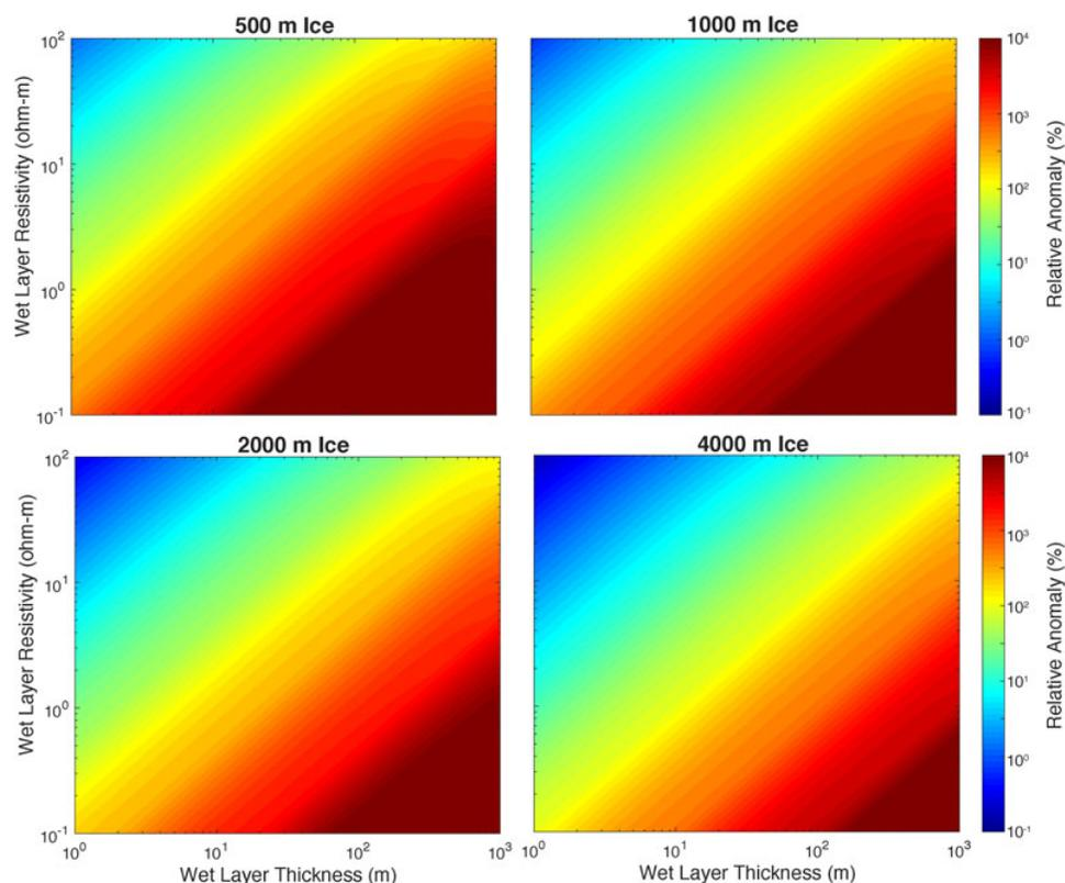
**Fig. 4.** Relative anomaly in the MT apparent resistivity response for a model with a conductive wet layer shown as a function of the layer resistivity and thickness. The anomaly is computed as the maximum relative difference between the response of the wet layer model and the response from a model without the wet layer. The maximum relative difference was computed in the frequency band 0.001–10 000 Hz and is shown for four different ice thicknesses (500, 1000, 2000 and 4000 m).
