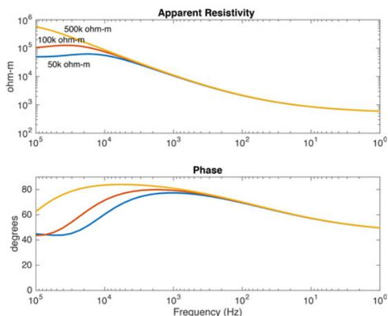
**Fig. 5.** Effect of ice resistivity on the MT impedance response for a 1D model with 1000 m thick ice overlying a 500  $\Omega$ -m halfspace. The variable ice resistivity affects only the high-frequency portion of the response.
