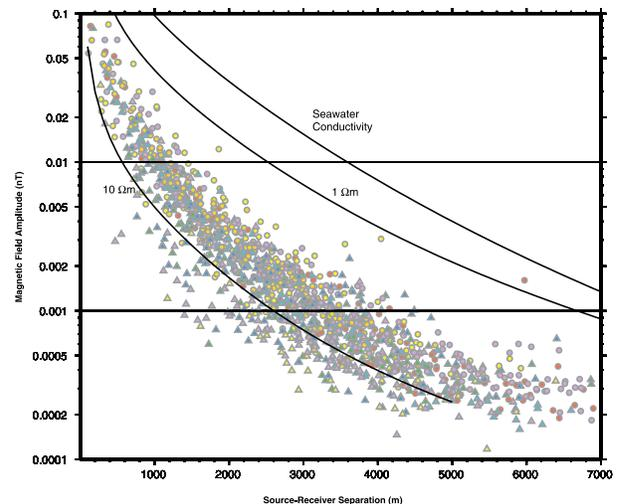
**Figure 2.** Magnetic field amplitude data for all instruments. Amplitudes for each receiver are shown using the same color symbol used for receiver location in Figure 1, with circles for the ridge crest instruments and triangles for those off-axis. If the underlying seafloor were a uniform layered structure, amplitudes from different receivers would plot along the same amplitude versus range curve. The effect of differing seafloor resistivity is shown by the 1/2 space curves as labelled.
