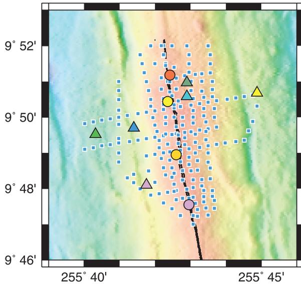
**Figure 1.** A map of bathymetry across the EPR at 9°50'N showing locations of our ten ocean bottom magnetometers (colored circles and triangles) and the more than 200 transmission stations (blue squares) completed during our experiment.
