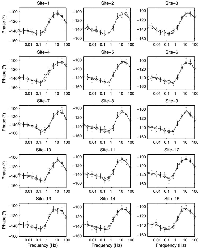
Figure 5. Comparison between the synthetic observed (solid lines) and calculated (dashed lines with circles) TM-mode phases using the model formed from the estimated medians of individual parameters. The vertical segments show the 95% error bars around data.
